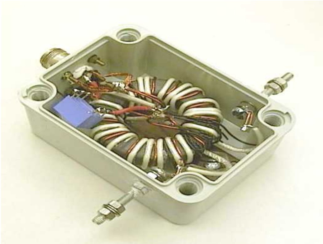
Fig.3 Photo of the balun showing construction details
